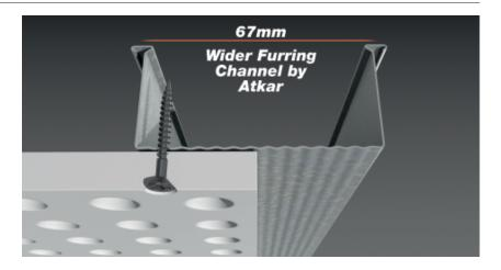
Screws should be spaced no more than 170mm from each fixing point and the distance between screw and panel edge is not to exceed 26mm.
