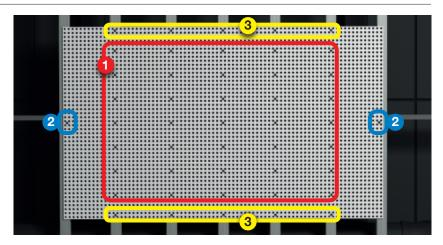
Panels come with printing on one edge and it is important that they are all installed with the printing facing the same direction.
