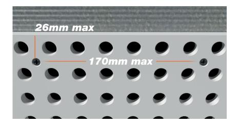
To secure the panel, first screw into the centre section of the panel (1), followed by the centre of each short edge (2) before finally screwing down the long edges (3) as per the diagram.
