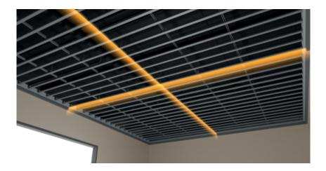
For best panel arrangement, locate the centre of the room, then lift the first panel into position.
